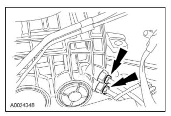
5. Remove both transmission fluid cooler tube quick connect secondary latches.
