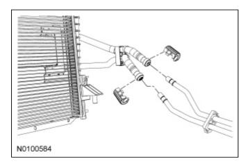
4. NOTE: Use a backup wrench to hold the case fitting secure.
