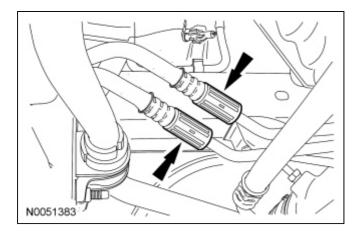
6. Using the Transmission Cooler Line Disconnect Tool, disconnect both transmission cooler tubes from the transmission fluid cooler hoses.
